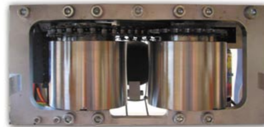
Loud squash ball cannon that fires balls at approx. 50km/h.
